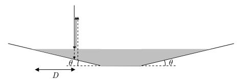
A beam that falls on the oil surface can either reflect straight back (solid arrow) or go through the oil, reflect from the dish and then back up through the oil (dotted arrow). Since the dotted beam has travelled longer than the solid beam, they interfere.
